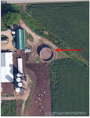
Figure 2. An older empty circular manure storage structure
